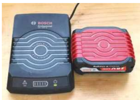
▲ The charger and battery with their distinctive markings. Note circular recess on charger
